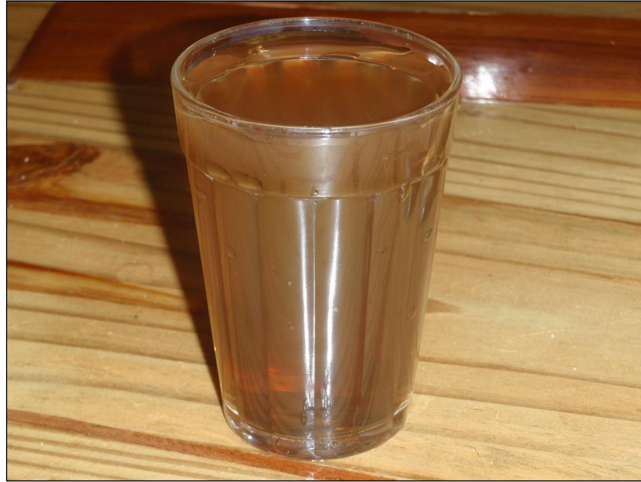
Identical color in water from hand-dug wells in village of Santa Rita (after addition of bleach)
